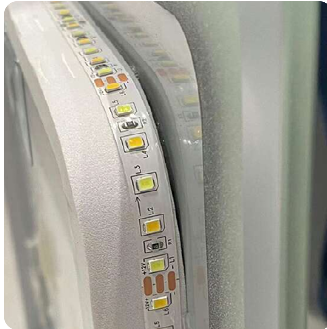
Foam strip and exposed light strip
